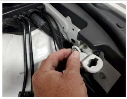
Remove the 13mm bolt in the driver side apron panel
