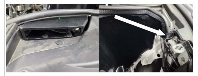
Lower heat shield into the area, secure the shield with the supplied push pins in the front scoop **FIRST** then use the supplied 13mm stainless bolt to secure to the side. Push in weather strip push pin into shield.
