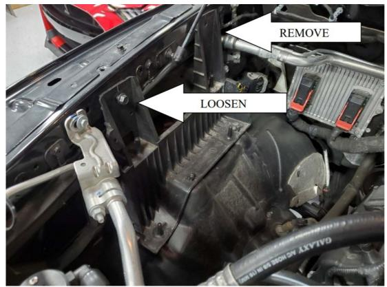
7. Slide JLT airbox into position with LOWER most locating pin in hole in the bottom of the shield Forward most TAB located BETWEEN fender and airbox mounting tab and rear most tab inside rear mounting hole
