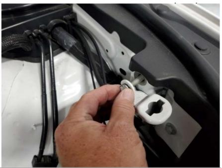
6. Lower heat shield into the area, secure the shield with the supplied push pins in the front scoop FIRST then use the supplied 13mm stainless bolt to secure to the side. Push in weather strip push pin into shield.
