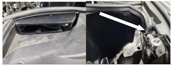
7. Lower air filter down into the airbox first, then with the silicone reducer on the tube with clamps loose, connect the tube and air filter then slide onto throttle body.
