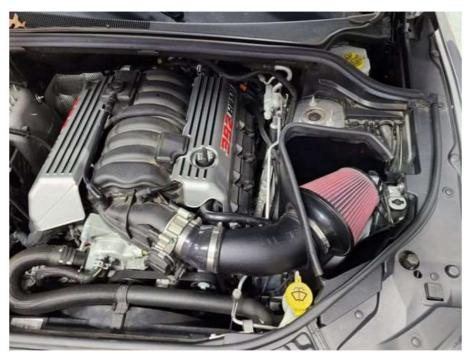
Oil Filter: The frequency you should clean your filter will depend on your driving conditions. It is recommended to check your filter at every oil change or 3,000 miles. If there is a buildup of dirt as thick as the wire mesh, then it's time to clean your filter.
