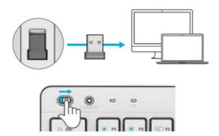
If connection is unsuccessful, hold Connect until purple LED flashes quickly. Unplug and re-plug dongle into computer.
