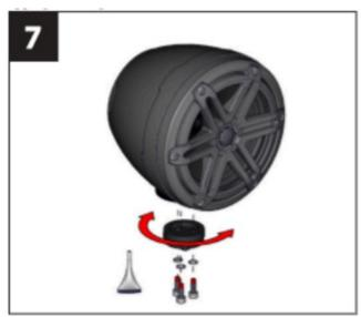
8. Align the keys of the Mounting Base with the keyways in the Mounting Receiver, then in sert fully. Aim the speaker in the desired direction, and tighten the Set Screw in the Mounting Receiver. Remove adhesive
