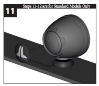
12. Gently press on the appliqué from the center out to remove any air pockets.
