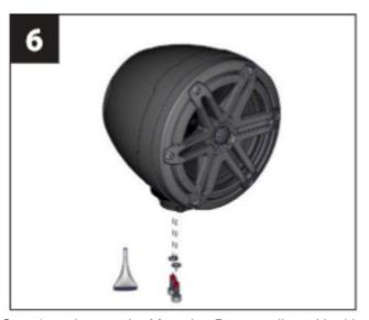
7. Remove the fasteners from Step 1, and rotate the Mounting Base to align with either the next or previous mounting hole in the Fixture Base. Slide a Split Lock Washer over each of three M6 x 16 mm Socket Cap Machine Screws, apply Loctite\* Red Thread Locking Compound to the screws, and fully tighten into the Fixture Base.
