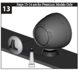
14. Align the aluminum logo cap to the desired angle of rotation, and press it onto the back of the enclosure. Apply masking tape (not included) to hold the cap in place until the silicone cures (at least 24 hours).
