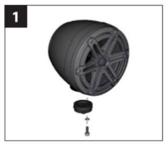
2. Partially thread the M6 x 20 mm Set Screw into the Mounting Receiver. Align the keys of the Mounting Base with the keyways in the Mounting Receiver, then insert fully.
