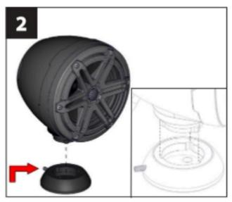
3. Place the enclo sure at its desired location with the speaker and Set Screw aimed in the desired direction. L'se a pencil to draw an outline of the Mounting Receiver's base and location of the Set Screw on the mounting surface. Next, while holding the Mounting Receiver with one hand, rotate and pull the enclosure away to separate it.
