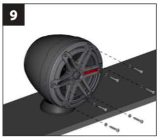
10. Rotate the speaker to the desired angle. Reinstall the speaker and speaker mounting screws and washers. Hand-tighten in a criss-cross pattern.
