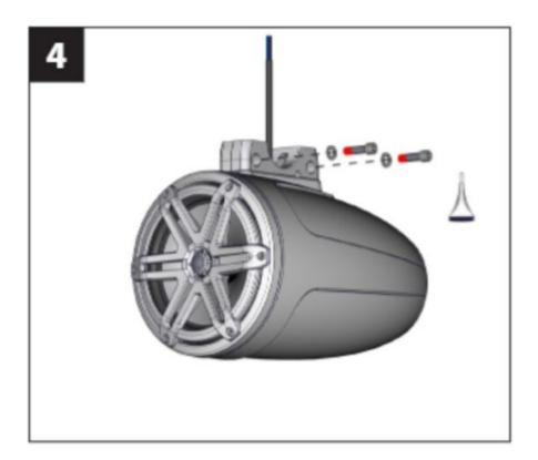
Align the Lower Fixture to the enclosure. Install (2) 5/16 Split Lock Washers and (2) 5/16-181-1/4 Machine Screws as pictured. Apply Loctite Red Thread-Locking Compound to each screw end, thread them into the Lower Fixture, and fully tighten while pressing down on the Lower Fixture to ensure no gap.
