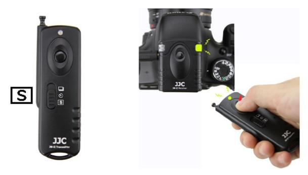
2. Then fully press while holding the shutter button of transmitter until the transmitter LED light OFF, and the receiver will now lock the shutter for continuous shot.
