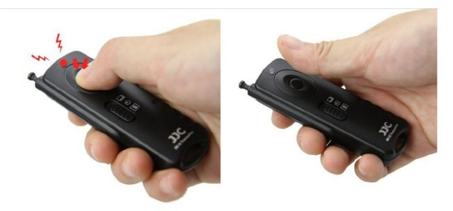
3. To release the shutter lock, press the shutter button of the transmitter again, and the receiver will unlock the shutter. Then you will get plenty of pictures.
