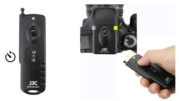
2. Then fully press the shutter button, and the camera will take a picture after 5 seconds count down. You will get a delay shot photo.
