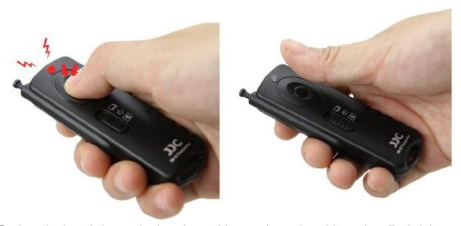
3. To release the shutter lock, press the shutter button of the transmitter again, and the receiver will unlock the shutter. Then you will get a long exposure photo as the picture shown below.
