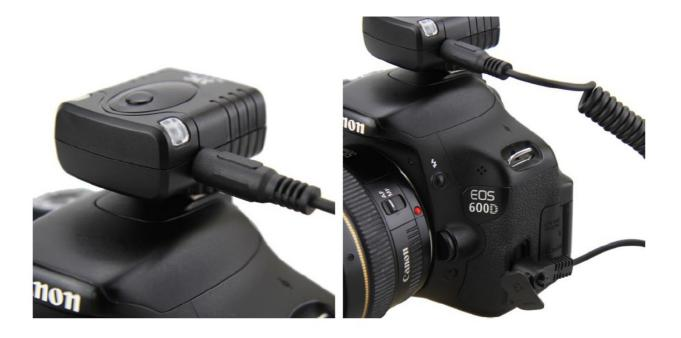
**Note:** Please remember not to connect the cable round the wrong way. For any JJC connecting cord, please always keep in mind that the end as the picture shown left should be plugged to receiver while the other end is for the camera remote socket.
