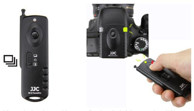
2. Then fully press the shutter button, and the camera will continuously take 3 pictures at an interval of 1s.
