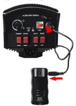
5. Turn on your camera, flash, and shift the Mode switch on receiver to the Flash option. Then press the shutter button on your camera, and both indicators on the transmitter and the receiver will turn green. At this time, your flash will be triggered successfully.
