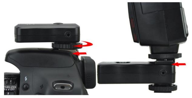
4. If your flash or studio light does not have a hot shoe, connect the flash or studio light with the ACC2 socket of the receiver by the studio light cable supplied in the package.
