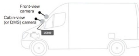
Figure 3-2 Installation Diagram of Front-view camera and cabin-view (or DMS) camera
