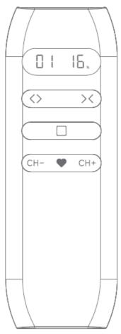
• JCH35W3C2 16-channel dual control LCD remote controller.
