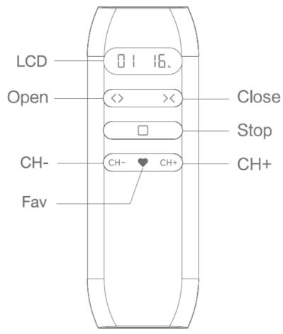
• JCH35W3C2 16-channel dual control LCD remote controller.
