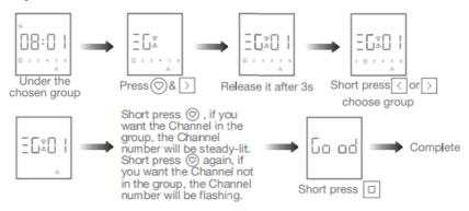
**Note:** Max&Min number is 6&1 when it's set under channel 0. Check the Channels in Groups
