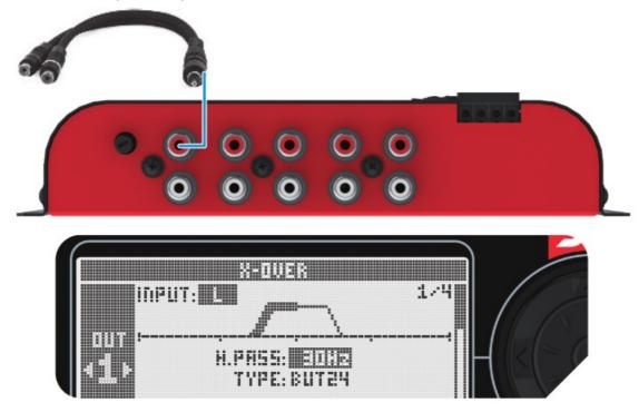
2. Put the player to play at a volume close to maximum, and keep the adjustment of the input gain as much as possible, without lighting the input clipping led.
