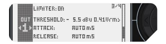
**ATTACK** – Is the response time of Limiter. When in AUTO (recommended), the time is defined as follows:
