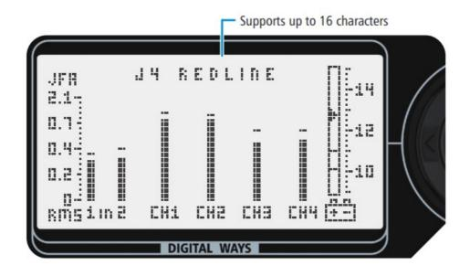
By pressing for 5 seconds on the level meter screen, enter the display text setting. To exit, simply press the centre key.
