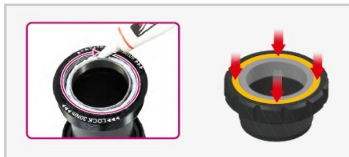
2. Ensure that the internal cable routing of the frame will not interfere with the bottom bracket (BB) installation. Clean the inside of the BB shell on the frame, ensuring it is smooth and free of debris. Apply a thin layer of grease to the inner edges of the BB shell to assist with smooth BB installation.
