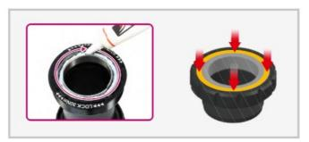
2. Ensure that the internal cable routing of the frame will not interfere with the bottom bracket (BB) installation. Clean the inside of the BB shell on the frame, ensuring it is smooth and free of debris. Apply a thin layer of grease to the inner edges of the BB shell to assist with smooth BB installation.
