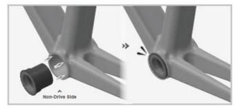
5. Align the drive-side BB along with the Snug Ring vertically with the inside of the drive-side BB shell on the frame, and rotate it counterclockwise to insert. Then, use the BB wrench (B015) to fit the drive-side BB, continuing to rotate counterclockwise to press it in. Tighten to a torque value of 30Nm, ensuring there is no gap between the BB and the frame's BB shell, completing the BB installation.
