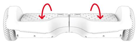
TO MOVE FORWARD: APPLY EQUAL PRESSURE TO THE FRONT OF EACH FOOTPAD WITH YOUR TOES.
