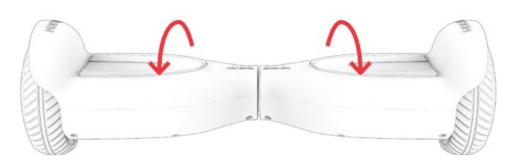
TO MOVE BACKWARDS: APPLY EQUAL PRESSURE TO THE BACK OF EACH FOOTPAD WITH YOUR HEELS.
