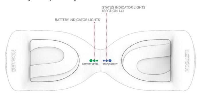
WHEN POWERED ON FOR USE, BATTERY INDICATOR LIGHTS WILL ILLUMINATE TO INDICATE CHARGE PERCENTAGES AS INDICATED IN THE TABLE BELOW.
