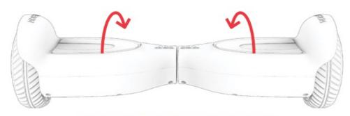
TO MOVE FORWARD: APPLY EQUAL PRESSURE TO THE FRONT OF EACH FOOTPAD WITH YOUR TOES.
