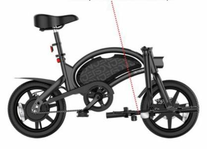
Press the Stem Quick Release in to lock position. To fold, unlock the Stem Quick Release.
