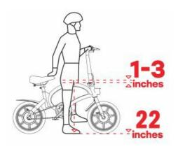
For safe and comfortable riding there should be a clearance of 22 inches from ground to the crotch of the intended rider. Also, at least 1-3 inches between the crotch and the top tube of the bicycle frame, while the rider straddles the bicycle with both feed flat on the ground. Women can use a men's style bicycle to determine the correct size women's model.
