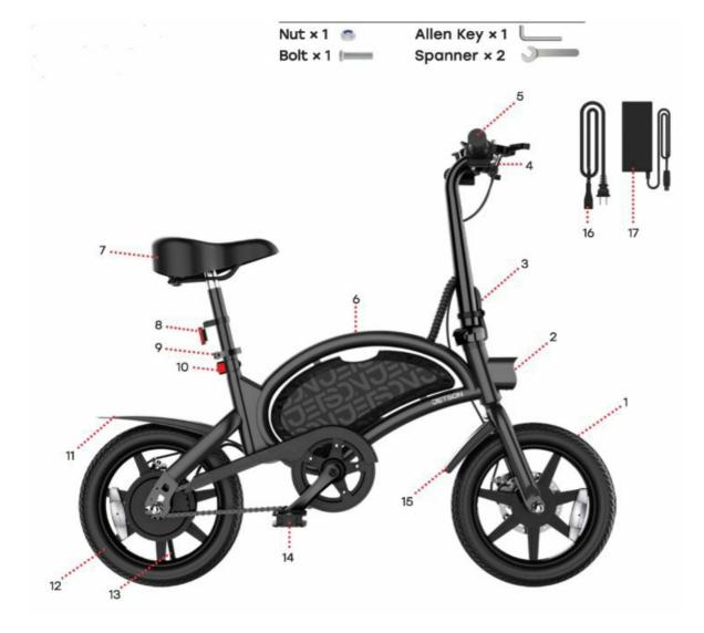
Tools needed but not included: Screw Driver, Ratchet + Socket **CAUTION**: Before operating the Bolt Pro please tighten all screws, nuts, and bolts.
