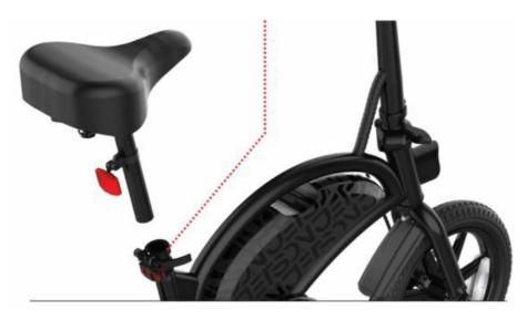
Turn the Knob clockwise to tighten Seat Clamp . Close the Seat Clamp
