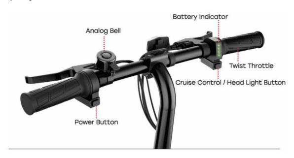
Power Button: Turns the Bolt Pro on and off .
