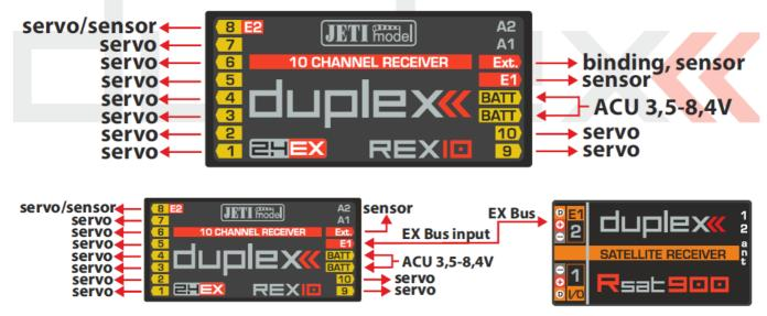
Note: the connection method of the satellite receiver RSAT900 and RSAT900NG are identical
