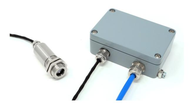
ExTempMini intrinsically safe non-contact infrared temperature sensors measure the temperature of an area of the surface of a solid or liquid, and transmit this as a linear 4-20 mA output.
