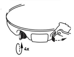
6. OPEN VALVE FULLY COUNTERCLOCKWISE AND FLIP IGNITER LEVER
