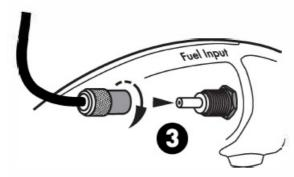
3. CONNECT AND SECURE REGULATOR TO FUEL INPUT PORT(REAR LEFT STOVE)
