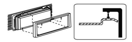
NOTE: For proper operation of the CD/DVD player, the chassis must be mounted within 30° of horizontal. Make sure the unit is mounted within this limitation.
