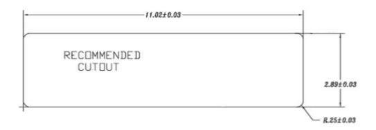
**NOTE**: Before cutting the mounting hole, make sure the area behind the mounting location is clear of wires, fuel and vacuum or brake lines.
