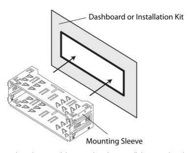
Step 2: Bend multiple mounting tabs around the mounting sleeve until the mounting sleeve is secure.
