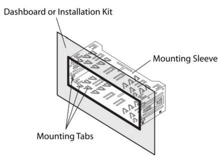
Step 3: Connect all wiring harnesses and slide the head unit into the mounting sleeve until it clicks into place.
