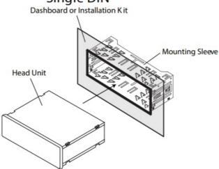
Mounting the Head Unit: ISO mounting
