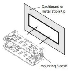
Step 2: Bend multiple mounting tabs around the mounting sleeve until the mounting sleeve is secure.
