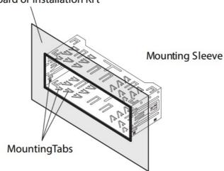
Step 3: Connect all wiring harnesses and slide the head unit into the mounting sleeve until it clicks into place.
