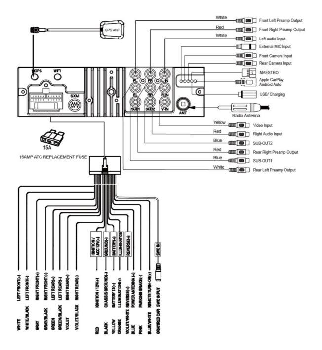
**Note:** When replacing a fuse, make sure to use the correct type and amperage. Using an incorrect fuse coul ause damage. The unit uses (1) 15 amp ATC mini style fuse located on the power connector
