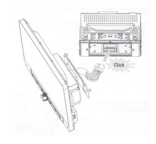
Use the hinge hooks on the back of the monitor to hold the LCD in place. Proceed to Step #4 to secure the LCD to the chassis.
