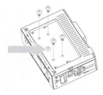
Depending on your vehicle's dash. the LCD mounting bracket can be adjusted to 3 positions (Flush .1 /2" and 1 "). The bracket comes in the Flush setting when purchased. To adjust the bracket to either the 1/2" or 1" setting, gently pull the LCD bracket out from the chassis. adjust it to the desired position and lock it in place by inserting the screws to the top of the chassis. (see below images for reference)
