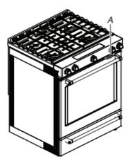
• Model/serial/rating plate (located behind the oven door on the top right-hand side of the oven frame)
