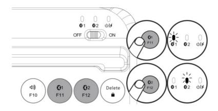
After bluetooth connected, short press " 1" or " 2" to easily switch between multiple devices.
