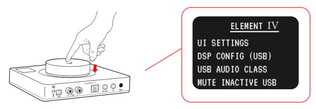
Pressing down on the Volume Knob for 3+ seconds enters the Options Menu. Turn the knob to navigate up/down the options menu. Push the knob to make a selection. For best experience, we recommend adjusting settings through Core. You will find up-to descriptions of each option and feature within Core.
