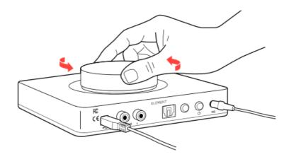
Pressing the volume knob toggles between USB and Optical input.
