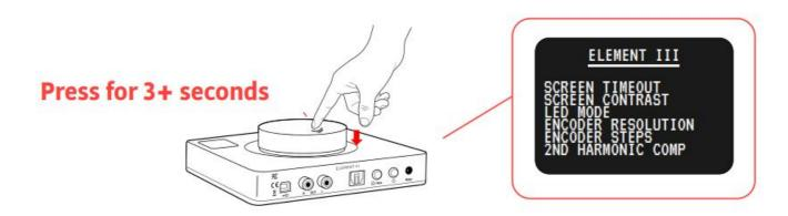
Pressing down on the Volume Knob for 3+ seconds enters the Options Menu (show below). Turn the knob to navigate up/down the options menu. Push the knob to make a selection.
