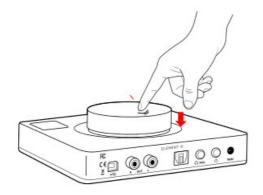
Pressing the volume knob toggles between USB and Optical input. Please see Connectivity and Computer Setup for additional help.
