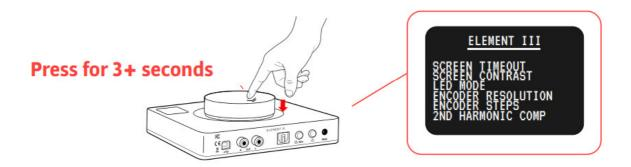
Pressing down on the Volume Knob for 3+ seconds enters the Options Menu (shown below). Turn the knob to navigate up/down the options menu. Push the knob to make a selection. Available settings are described below, with default values in **bold**.
