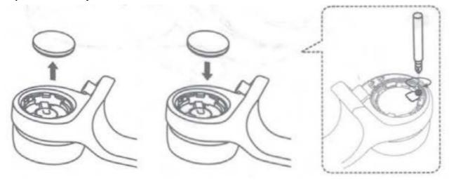
\* Change the battery when the LED starts flashing fast (4Hz)
