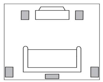
Some newer surround sound formats utilize left and right surround channels that are used for side fill, in additionto the left and right rear channels found in 5.1 systems. Place the left and right surround speakers on the sides of the room, at or in front of the listening position, facing each other.
