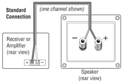
**IMPORTANT:** Do not reverse polarities (i.e., + to - or - to +) when making connections. Doing so will cause poor imaging and diminished bass response
