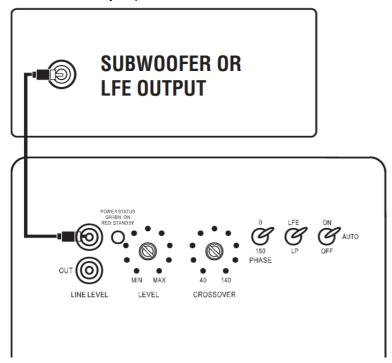
The 1500 Array includes a line output. This output allows you to "daisy chain" one 1500 Array to multiple 1500 Array subwoofers. Simply connect the first subwoofer as described above and then run a subwoofer cable from the line output(s) to the line input on the next sub
