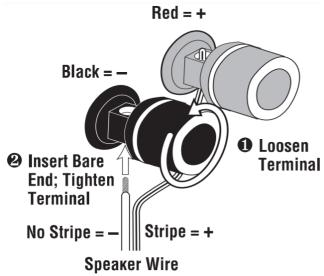
To ensure proper polarity, connect each + terminal on the back of the amplifier or receiver to the respective + (red) terminal on each speaker, as shown in **Figure 2.** Connect the – (black) terminals in a similar way. See the owner's guides that were included with your amplifier, receiver and television to confirm connection procedures.
