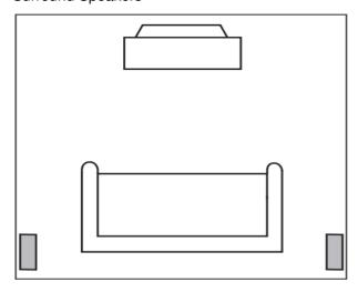
The front speakers should beplaced the same distance from each other as they are from the listening position, with tweeters at about the same height from the floor as the listeners' ears will be.
