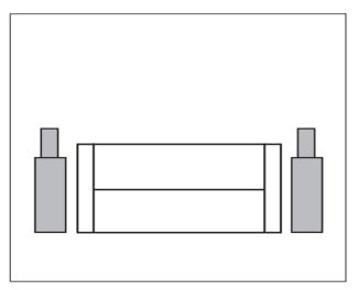
A 6.1-channel system will consist of a 5.1-channel configuration, as shown, with the addition of a rear center speaker placed midway between the two surround speakers, and further to the rear than the surrounds. The rear center speaker should not call more attention to itself than the surround speakers.
