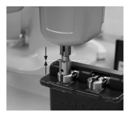
Adjust the Soldering Head position until the upper and lower centering jigs are aligned. It must be possible to move in and out smoothly.
