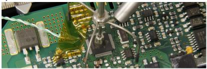
IPC\* does not recommend exceeding ramp-up rates over 3-4 °C / sec (5-7 °F / sec) so as to reduce the risk of thermal stress on the PCB. IPC was founded in the U.S. in 1957 as the Institute for Printed Circuits.
