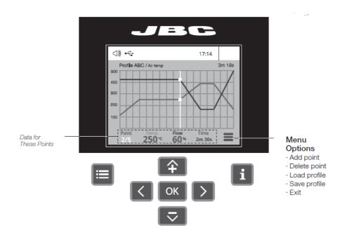
By pressing Graphics in the main MENU, temperature and power figures in real time are displayed. This helps you decide which tip to use to obtain the best quality solder joints.
