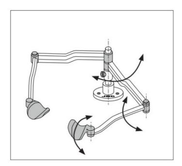
RHTD allows adjustment for different positions according to your work needs.
