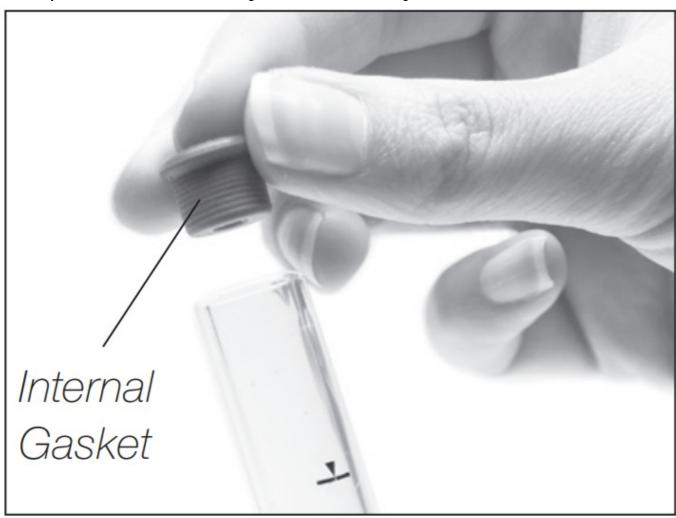
For a proper connection, it is essential to insert the cartridge so that it aligns with the mark
