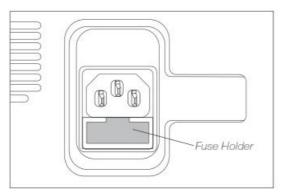
• Insert the new fuse into the holder and return it to the station.
