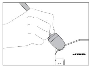
When the tool is in the stand, the temperature falls to the preset Sleep temperature.
