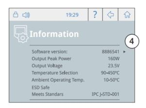
Select "Information" (3) and than press (4) to check the firmware version. For DDE / HDE / NAE / JTSE / TESE / ACE Preheater Console:
