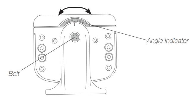
Note the angle indicator around the bolt area. Tighten the bolt for holding the body in the desired position. The soldering head must be set to the same angle.
