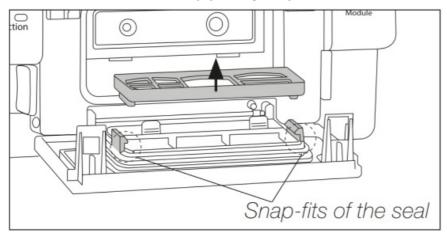
3. Position the new filter with its clear side upwards and with the cross-shaped strud at the left side
