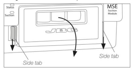
2. Remove the worn filter by pulling it upwards out of the snap-fits.
