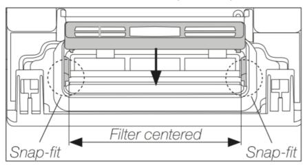
5. Push the positioned filter back until it stops against the transparent ribs.
