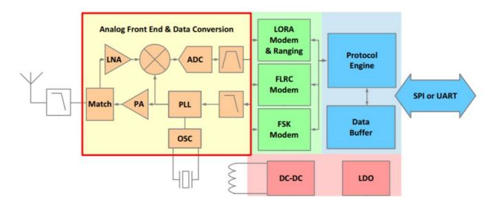
The modem uses spread spectrum modulation and Forward Error Correction (FEC) techniques to increase the range and robustness of radio communication links.
