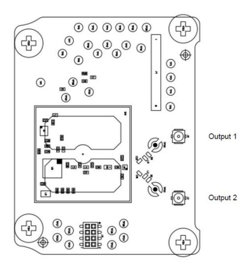
Antennas numbers 1, 2, and 3 can be connected directly to connector UFL on the radio board module. For antennas 4, 5, 6, and 7 it is necessary to have adaptor UFL to SMA females for connected these.
