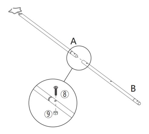
Screw the bolt into the small threaded hole to connect (A) with (B). STEP 2
