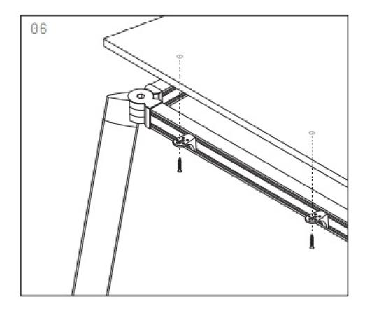
If this bolt does not drop into the joint use the Allen key to screw it all the way in so that it creates its own thread. This will ensure a nice, tight joint.
