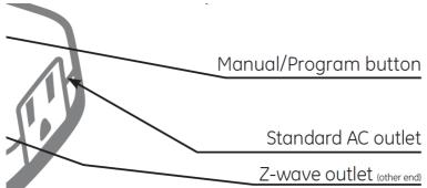
**CAUTION** — To reduce the risk of overheating and possible damage to other equipment, do not install to control a motor-operated appliance, a fluorescent lighting fixture, receptacle or a transformer supplied appliance.
