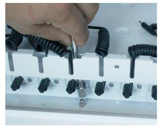
6. Position USB-C cables forward in the cable track so they are out of the way of the tray lid closing. Remove your prop from the side wall of the station and close the tray lid. Secure the tray lid shut using the screw and washer that were removed in step 2 with the Torx key.
