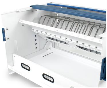
3. Remove the 3 nuts that secure the front panel of the tray to the bottom panel using the box wrench. Put the nuts in a secure location to secure the hub onto the tray later. Remove the front panel of the tray and set aside. You will not need this piece for the USB-C configuration.
