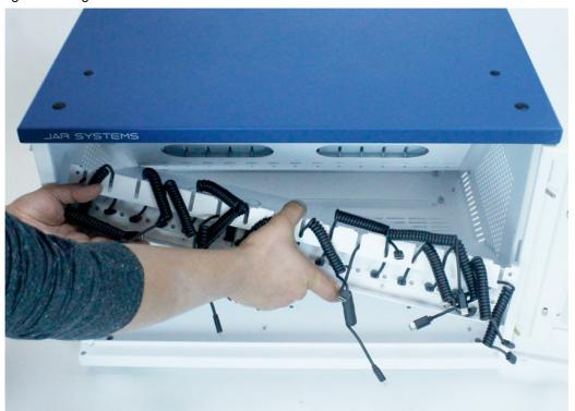
5. Align the holes in the front of the hub with the studs where the front panel was secured. Use the nuts that were removed in step 3 to secure the hub to the tray using the box wrench.
