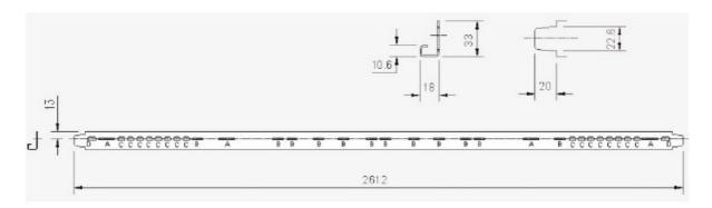
This Long Bracket is effectively used to support the detector and increase its overall length so that it can be secured to the top of the elevator car. The detector is secured to the Long Bracket by using the M3.5 nuts, bolts and washers provided in the fixing kit.
