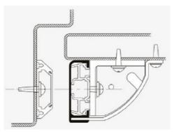
• 744 020 Self-Tapping Screw and standard fixing
