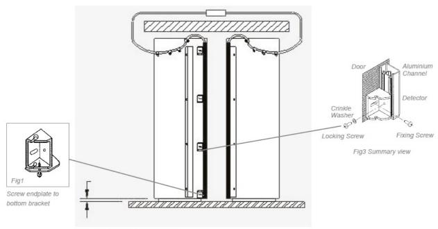
Fig2: Detectors Mounted on Doors
