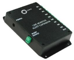
If the phone(s) are connected to an EMS5 Call Director, you should also use the Line Monitor Expansion Board (LMX) and connect the AUX1 of the EMS5 to any of the inputs of the LMX board and the ADA to the rest of the inputs.
