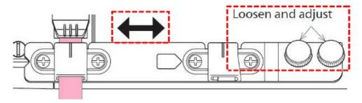
If the seam line seems out of alignment, adjust the Bias Tape Guide position by loosening the attachment screws.
