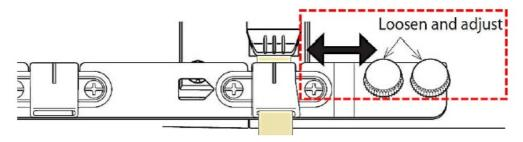
• If the seam line seems out of alignment, adjust the Belt Loop Folder position by loosening the attachment screws.
