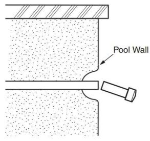
2. . Use Inside Pipe Cutter (part #5-17-4) to cut pipe back 5/8" behind shell surface.
